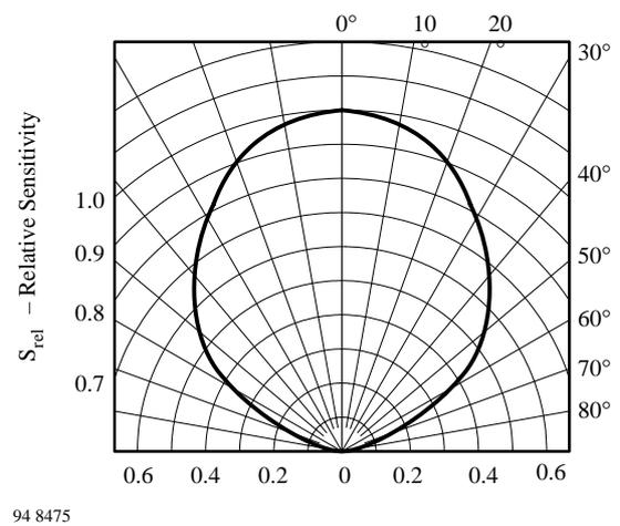
Figure 6. Relative Radiant Sensitivity vs. Angular Displacement
