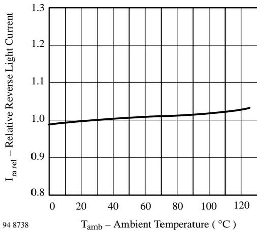
Figure 2. Relative Reverse Light Current vs. Ambient Temperature
